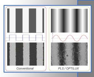
The here described system is equipped with the VIRELUX proprietary PLS light box design. It features a dedicated, sinusoidal profile light emission, improving operator ergonomy and visual accuracy.
